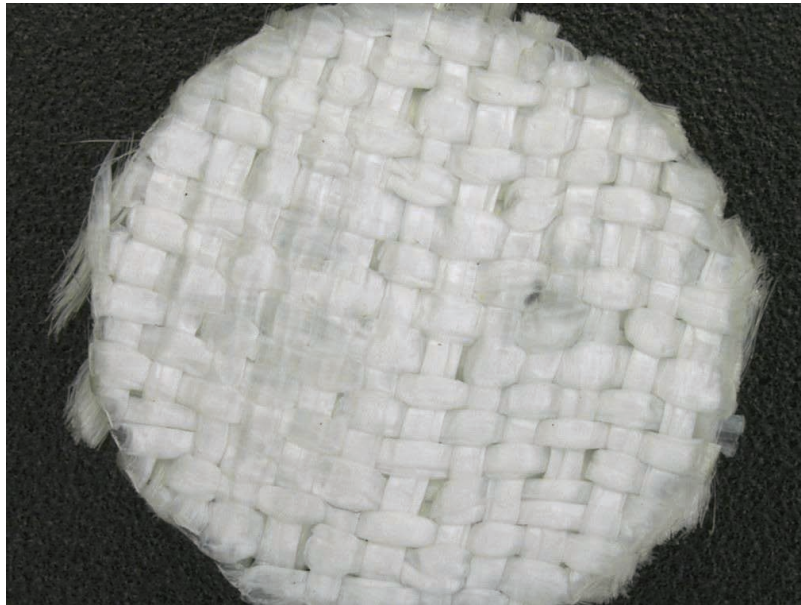
Coated Orthofabric prior to adhesion testing.
